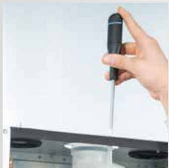
Removal of the stop screw of the smoke manifold
